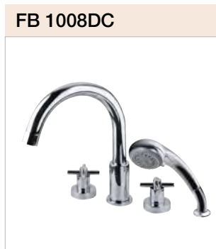
Bathtub faucet (hole : two handle Ø37-40, spout : Ø35-38, shower head : Ø35) left side : hot right side : cold
