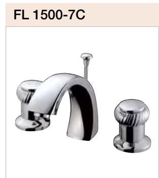
8" Lavatory faucet (hole : two handle Ø 35-38, spout : Ø30-32) left side : hot right side : cold
